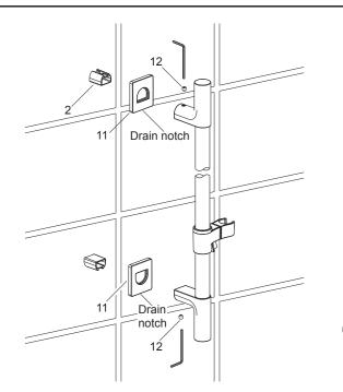
Slide the bracket escutcheons(11) onto the bases(2), confirm the drain notch of the escutcheon is pointed down. Install the whole slide bar onto the bases.
