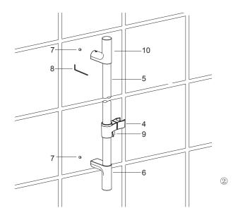
Place the bar(5) into the under slide bar body(6). Install the screw(7), tighten them by hex wrench(8).
